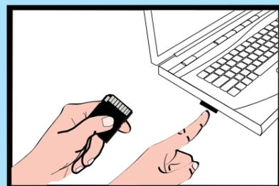
Insert the SD card into the SD card reader and connect the card reader, to your computer. A window will pop-up. Please run the "install.exe". Provide the necessary data to proceed. Since you have completed this step simply remove the SD card reader and set the SD card into the **talk2lift®** device. The device will be automatically updated with the information that the user has provided. The system is now ready for use and is waiting for the voice commands.
